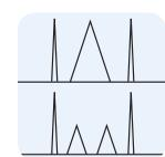
One of the major causes of inconsistent results is sampling and injection technique. Check that each sample is being injected the same way.
