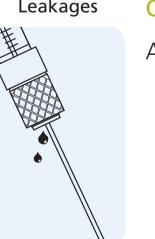
The needle may not be fitted correctly. Remove and refit the needle. Check needle seal is in place and undamaged.
