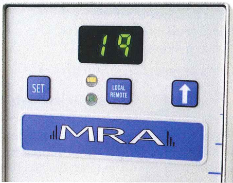
MRA in Local (manual) mode. Note indicator light for Local is illuminated. Split Factor of 19 is displayed by Split Factor LED.
