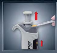
Remove the colour cap using the calibration key. Set the calibration switch in its upper position.
